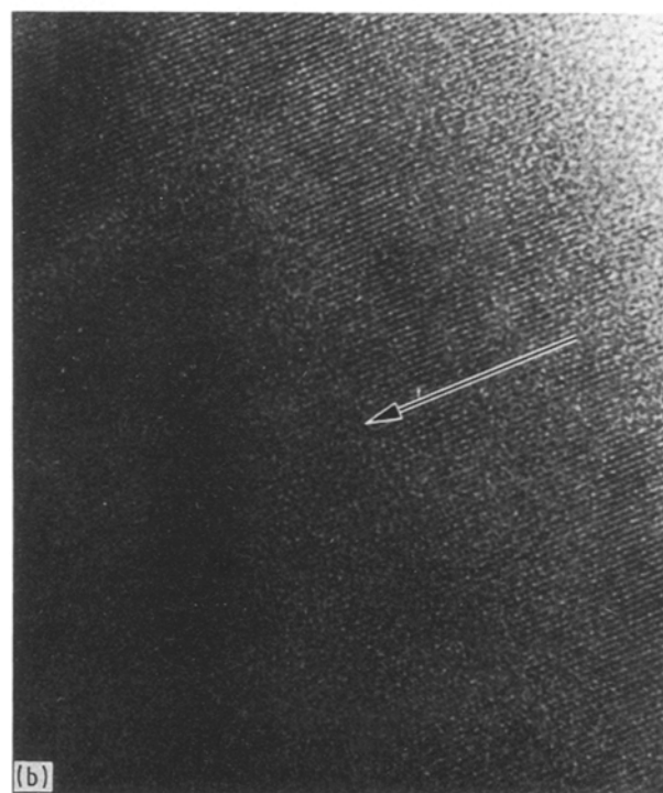
Figure 13 High-resolution transmission electron micrographs of a liquid phase showing (a) the lattice fringes in the liquid phase. (b) Higher magnification.
